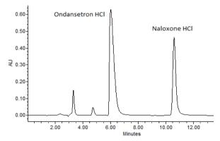
Fig. 1: High-performance liquid chromatography analysis of an injection combination containing ondansetron hydrochloride (0.4 mg/ml) and naloxone hydrochloride (0.2 mg/ml) in 0.9% water of injection (sodium chloride) after 24 hours storage at 37 °C
