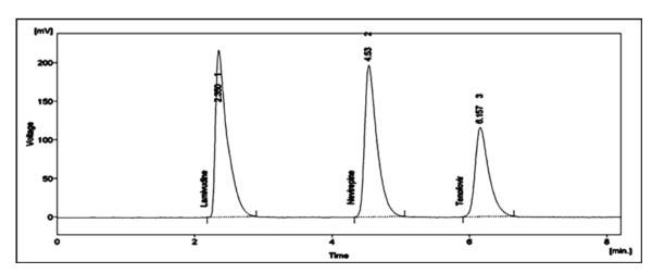
Fig. 2: Optimized chromatogram of the proposed method
