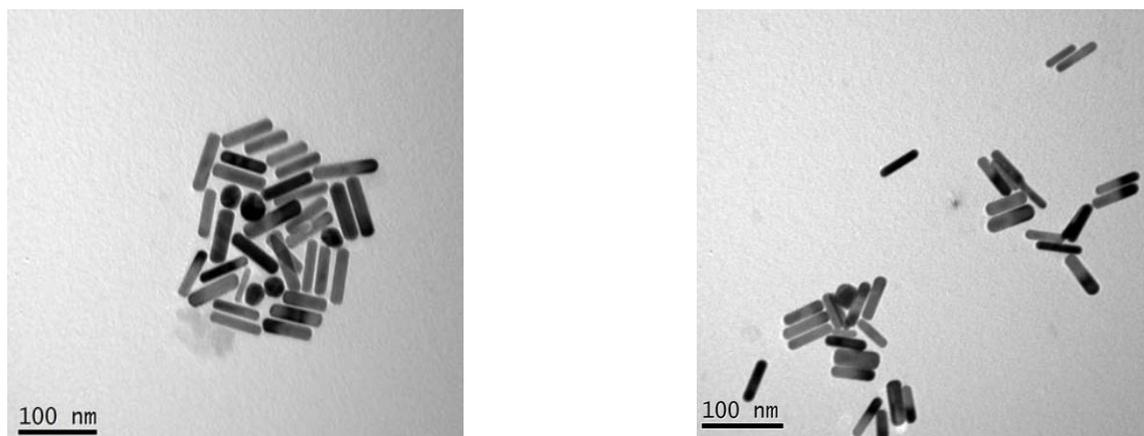
Fig. 1: TEM image of gold NRs with plasmon band energies at 800 nm
