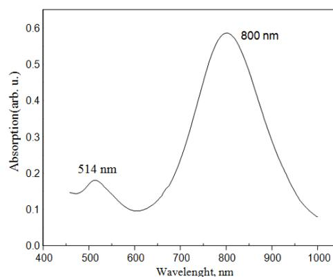
Fig. 2: UV-Visible-NIR absorption spectra of the gold NRs prepared using single surfactant mixtures
