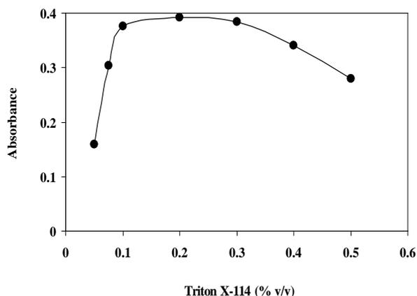
**Fig. 5: Effect of Triton X-114 surfactant concentration on the absorbance after CPE. Conditions: Co(II), 100 ng/ml; BTANP, ( $1.0 \times 10^{-4}$  mol/l) and pH 7.0. Other experimental conditions are described under procedures**
