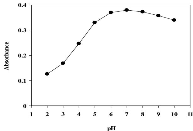
Fig. 3: Effect of pH on the absorbance after CPE. Conditions: Co (II), 200 ng/ml; BTANP, ( $1.0 \times 10^{-4}$  mol/l) and Triton X-114, 0.2% (v/v). Other experimental conditions are described under procedures
