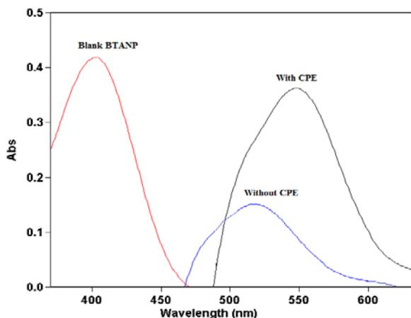
Fig. 2: Absorption spectrum of Co (II)-BTANP complex with and without CPE procedure against BTANP reagent blank
