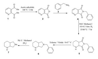
Scheme 1: Synthetic scheme for the preparation of octahydro-1*H*-pyrrolo [3,4-*b*]pyridine
