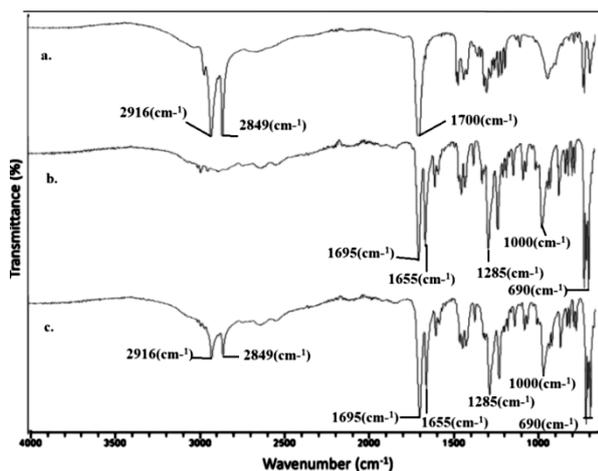
**Fig. 2: FTIR spectrum of (a) stearic acid, (b) pure drug and (c) KPF-Loaded-SLMs**
