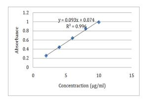
Fig. 2: Calibration curve of standard solutions (2-10 µg/ml)
