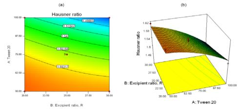
Fig. 7: Effect of independent factors on Hausner ratio (a) Contour plot and (b) Response surface plot
