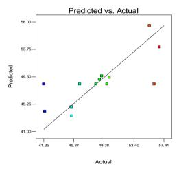
Fig. 1: Plot of actual versus predicted values for angle of repose
