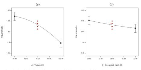
Fig. 6: Plot of individual effect of the quantity of (a) Tween 20 and (b) excipient ratio on Hausner ratio
