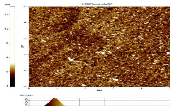
**Fig. 5: AFM image of GCBNP 3 nanoparticles**
