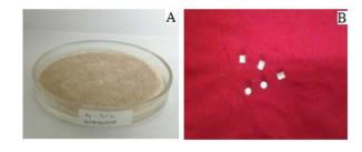
Fig. 2: Formulation process of bovine hydroxyapatite-chitosanciprofloxacin implants using glutaraldehyde, A) dry granules, B) implants (cylindrical pellets)
