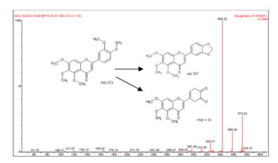
Fig. 2: Fragmentation ion mass spectra of sinensetin
