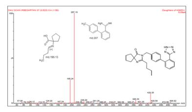
Fig. 1: Fragmentation of ion mass spectra of irbesartan
