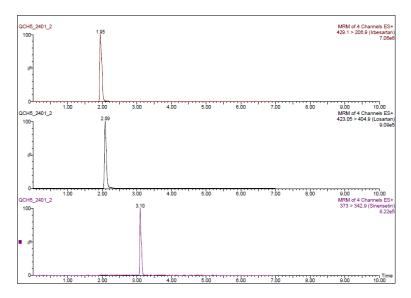
Fig. 3: Chromatogram of irbesartan, sinensetin and losartan simultaneously
