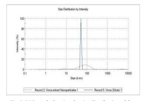
Fig. 3: DLS graph showing the size distribution of the nanoparticles for a fresh and a week old sample
