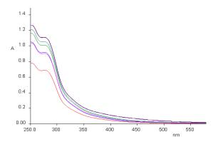
Fig. 2: UV-Vis Spectra of *Vinca* leaf extract and AgNO<sub>3</sub> solution reaction mixture
