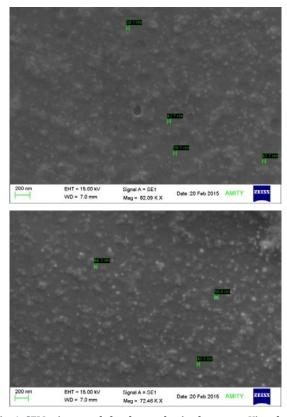
Fig. 4: SEM micrograph for the synthesised aqueous Vinca leaf extracts silver nanoparticles
