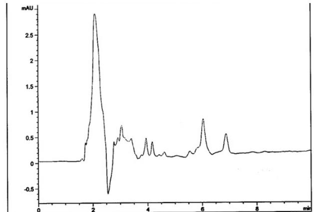
Fig.12: HPLC analysis of blood sample following administration of budesonide microspheres (after 2h)
