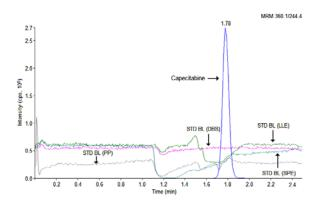
Fig. 4: Comparison of extraction techniques (LLE, PP, SPE and DBS) for matrix effect by post-column infusion technique
