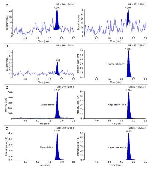
Fig. 3: MRM ion chromatograms of (A) double blank plasma (without analyte and IS), (B) blank plasma and capecitabine-d11 (IS) (m/z 371.2  $\rightarrow$  255.2), (C) capecitabine (m/z 360.2  $\rightarrow$  244.2) at LLOQ and IS, (D) Capecitabine (m/z 360.2  $\rightarrow$  244.2) at ULOQ and IS
