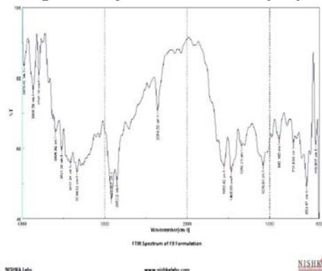
Fig. 5: FTIR spectra of formulation (F9)
