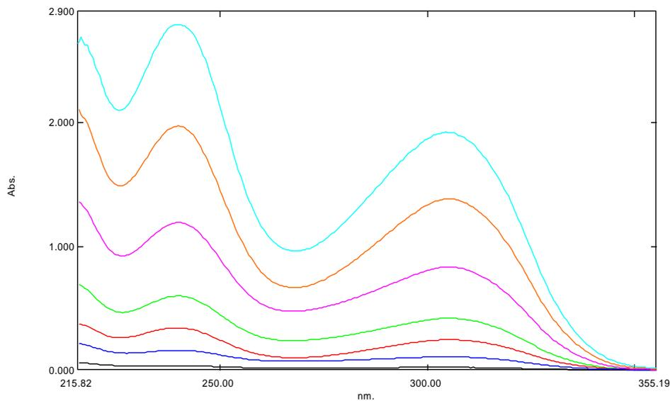
Fig. 2A: Absorption spectrum of CTB in 0.1 N HCl
