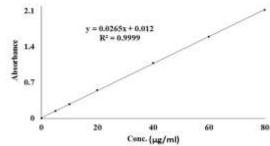
Fig. 3C: Calibration curve of CTB in phosphate buffer (pH 7.0)
