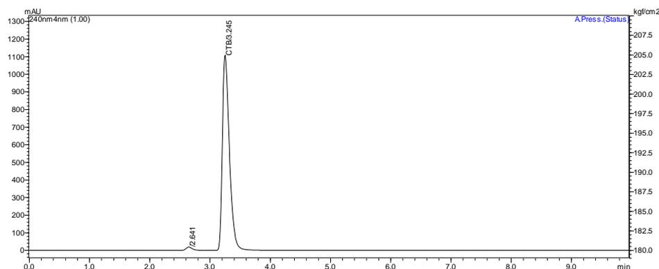
Fig. 4F: Typical chromatogram of protolytic degradation of CTB
