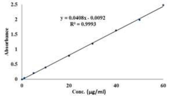
Fig. 3D: Calibration curve of CTB in borate buffer (pH 9.0)
