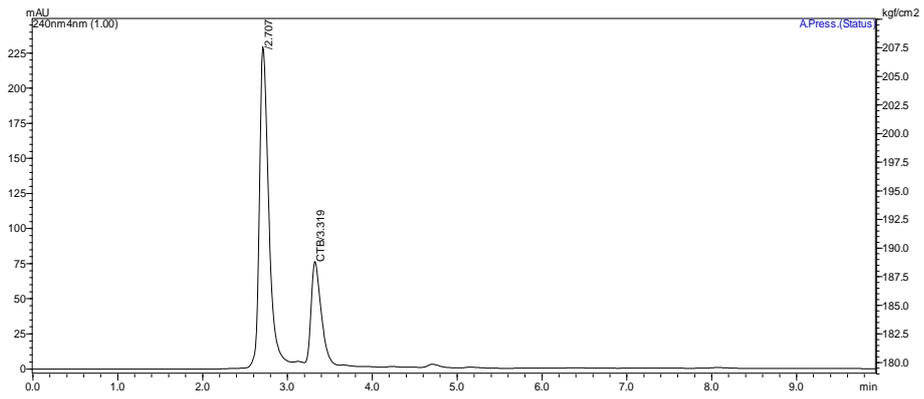
**Fig. 4B: Typical chromatogram of acid degradation of CTB**
