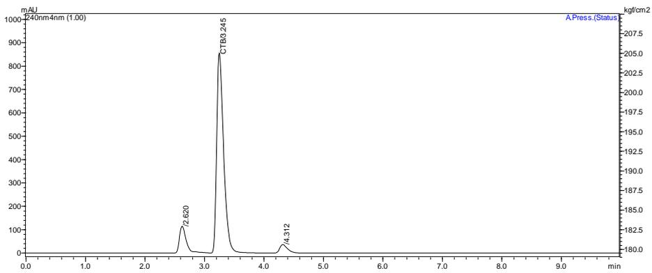
**Fig. 4D: Typical chromatogram of thermal degradation of CTB**
