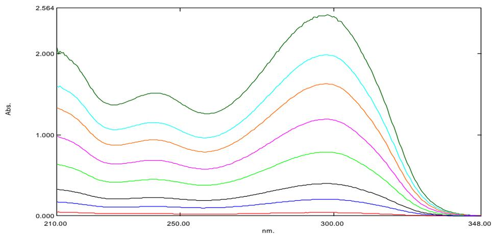
Fig. 2D: Absorption spectrum of CTB in borate buffer (pH 9.0)
