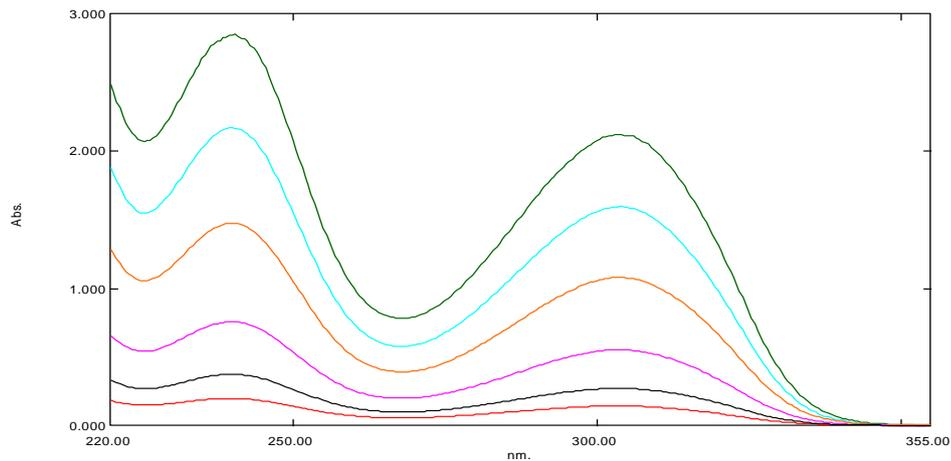
Fig. 2C: Absorption spectrum of CTB in phosphate buffer (pH 7.0)
