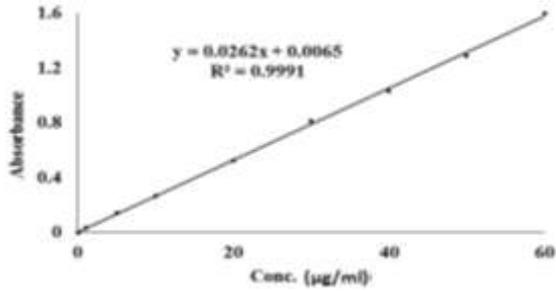
Fig. 3B: Calibration curve of CTB in sodium acetate buffer (pH 4.0)
