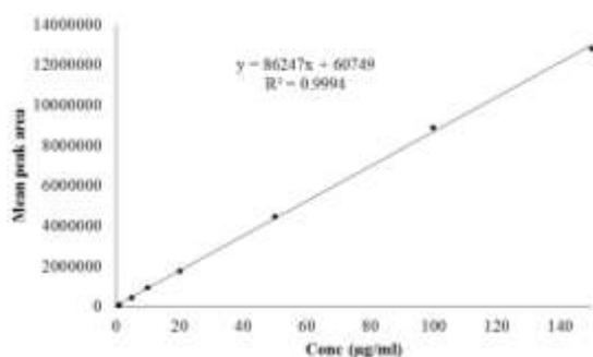
Fig. 5: Calibration curve of CTB in 0.1% acetic acid: acetonitrile
