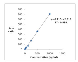
Fig. 5: Spiked concentrations (2ng/ml to1000ng/ml) were plotted against peak area ratio Vs Concentration with nine point calibration used for quantification by linear regression
