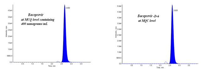
Fig. 3: Representative MQC-chromatograms of boceprevir and its internal standard
