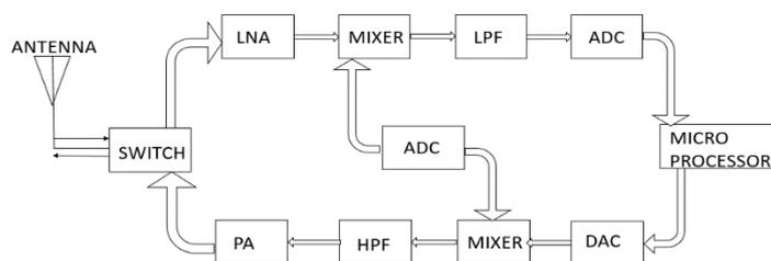
**Fig. 2: Block diagram of a transmitter**
