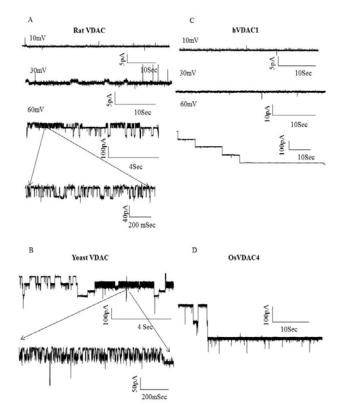
Fig. 2: Functional characterization of VDACs purified from different sources by using BLM. Current traces were observed in response to applied Voltage. (A) Rat VDAC starts transition from 30mV and shows many transitions at higher potential. (B) Yeast VDAC shows many transitions like rat VDAC. (C) hVDAC1 shows very few transitions at higher potential and that to from 60mV and above. (D) OsVDAC4 show very few transitions like hVDAC1.
