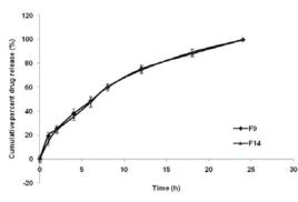
Fig. 6: Comparative dissolution profile of optimized NaCMC based optimized mini tablets (F9) and capsule filled with 25 number of mini tablets optimized formulation (F14)
