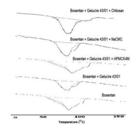
Fig. 2: Differential scanning calorimetry thermograms of bosentan and physical mixture (1:1) of drug with polymers
