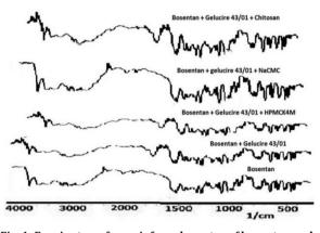
Fig. 1: Fourier transforms infrared spectra of bosentan and physical mixture (1:1) of drug with polymers
