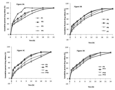
Fig. 3: *In vitro* dissolution profile of Mini tablets. (fig. 3A: Gelucire 43/01 based SR mini tablets, fig. 3B: HPMCK4M based mucoadhesive SR mini tablets, fig. 3C: NaCMC based mucoadhesive SR mini tablets and fig. 3B: Chitosan-based mucoadhesive SR mini tablets)
