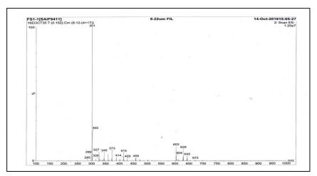
Fig. 4: Mass spectrum of compound FS-1
