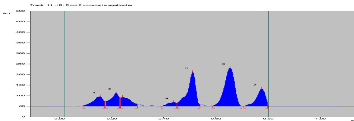
Fig. 5: HPTLC chromatogram of root extract has been shown under UV-254 nm wavelength
