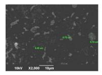
Fig. 3: SEM image of silver nanoparticles synthesized using rhizome extract of *Hedychium coronarium* at a concentration of 0.5 mM silver nitrate
