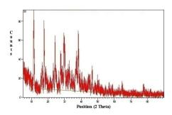
Fig. 4: X-ray diffraction pattern of silver nanoparticles synthesized using rhizome extract of *Hedychium coronarium* at a concentration of 0.5 mM silver nitrate.
