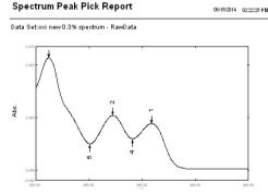
Fig. 5: Spectrum of oxidatively (0.3%) degraded MTD
