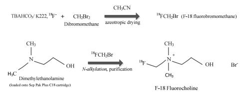
Fig. 1: Synthesis of F-18 fluorocholine
