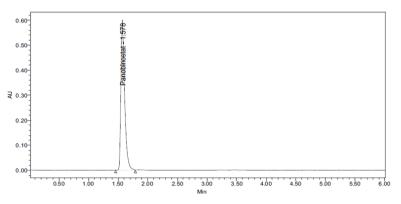
Fig. 6C: Peroxide degradation chromatogram
