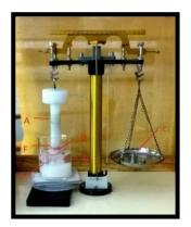
Fig. 1: Modified mucoadhesion test apparatus (Fabricated)
