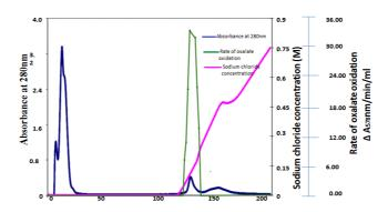
Fig. 4: Anion exchange chromatography of oxalate oxidase. ASF concentarted oxalate oxidase was purified using CM cellulose, cation exchange media and eluted with a 0 to 0.9M sodium chloride gradient. Protein content at A280 nm\* was monitered spectrophometric method. All fractions eluted (5 ml) were assayed using the MBTH assay at 590 nm\* in triplicate
