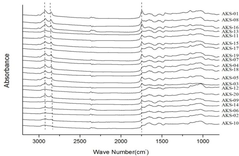
**Fig. 9: Comparative analysis of the FTIR absorbance spectra of isolated species in which absorbance at 2928, 2860 and 1740 cm<sup>-1</sup> shows the lipid content**
