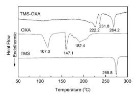
Fig. 3: Thermogram DTA of TMS-OXA co-crystal compared to its starting components
