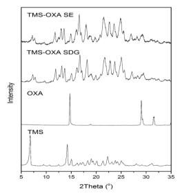
Fig. 2: PXRD patterns of TMS-OXA co-crystals prepared by solvent-drop grinding (SDG) and solvent evaporation (SE) compared to its starting components
