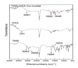
Fig. 4: FTIR spectra of TMS-OXA co-crystal compared to its starting components
