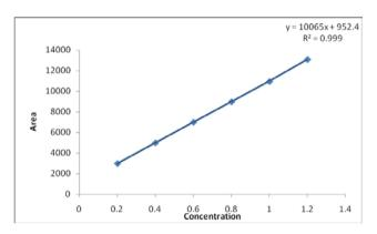
Fig. 3: Calibration curve of voglibose (0.2-1.2 µg/spot)
