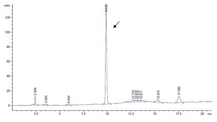
Fig. 3: HPLC-chromatogram of HES using UV-detector at wavelength of 280 nm
