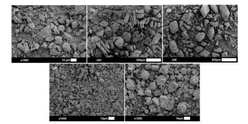
Fig. 6: SEM images of KTZ (a), FUMA (b), OXA (c), KTZ FUMA (d), KTZ OXA (e)
