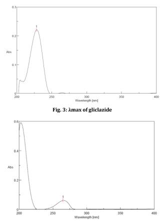
Fig. 4: λmax of sitagliptin phosphate monohydrate
