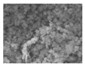
Fig. 1: SEM analysis of the synthesized mesoporous silica nanoparticles
