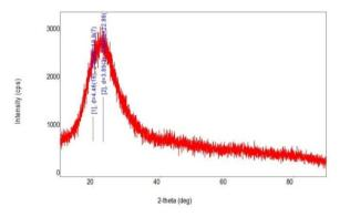
Fig. 3: Powder XRD-pattern of synthesized mesoporous silica nanoparticles
