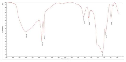
Fig. 4(c): FTIR spectra of tetracycline-loaded mesoporous silica nanoparticles
