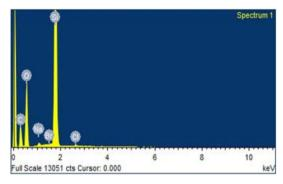
Fig. 2: EDS anylsis of synthesized mesoporous silica nanoparticles
