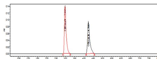
Fig. 4: Chromatogram of mixture of OFX and FLX under photolytic condition
