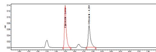
Fig. 7: Chromatogram of mixture of OFX and FLX degraded under alkaline conditions
