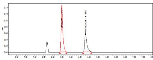
Fig. 6: Chromatogram of mixture of OFX and FLX degraded under acidic condition
