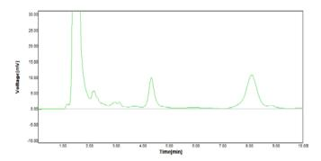
Fig. 2: Chromatogram of Deferasirox (4.8 µg/ml) in optimized chromatographic conditions
