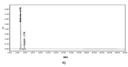
Fig. 3: Representative chromatograms of Acid (A), Base (B), Peroxide (C), Thermal (D), Photolytic (E) degradation of alogliptin and metformin
