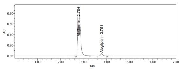
Fig. 2: A typical standard chromatogram of alogliptin benzoate and metformin hydrochloride
