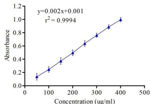
Fig. 4: Calibration curve of NFH in phosphate buffer, pH 7.4 using UV spectroscopy
