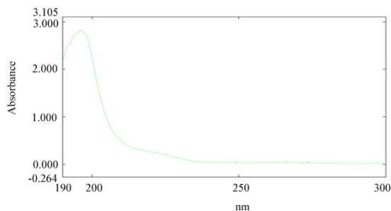
Fig. 2: UV scans of blank phosphate buffer, pH 7.4
