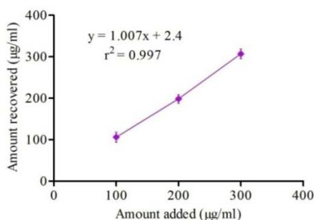
**Fig. 6: Graphical representation of accuracy****Table 4: Data for accuracy determination of UV spectrophotometry analytical procedure**
