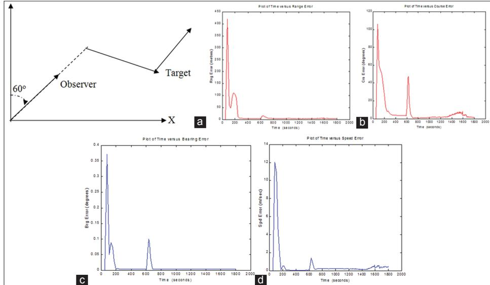
Fig. 3: Target motion analysis with single observation platform with target maneuver, with target maneuver (a) Error in range estimates, (b) error in course estimates, (c) error in bearing estimates, (d) error in speed estimates
