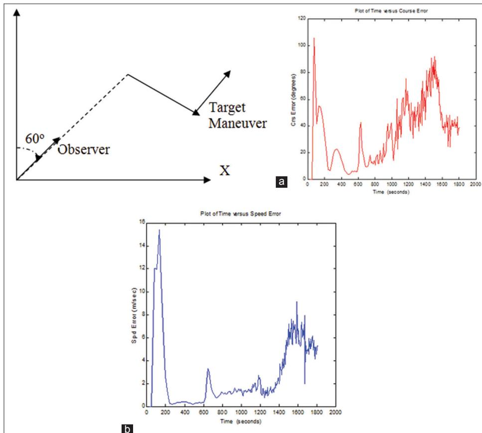
Fig. 4: Target motion analysis with single observation platform, (a) Error in course estimates, (b) error in speed estimates
