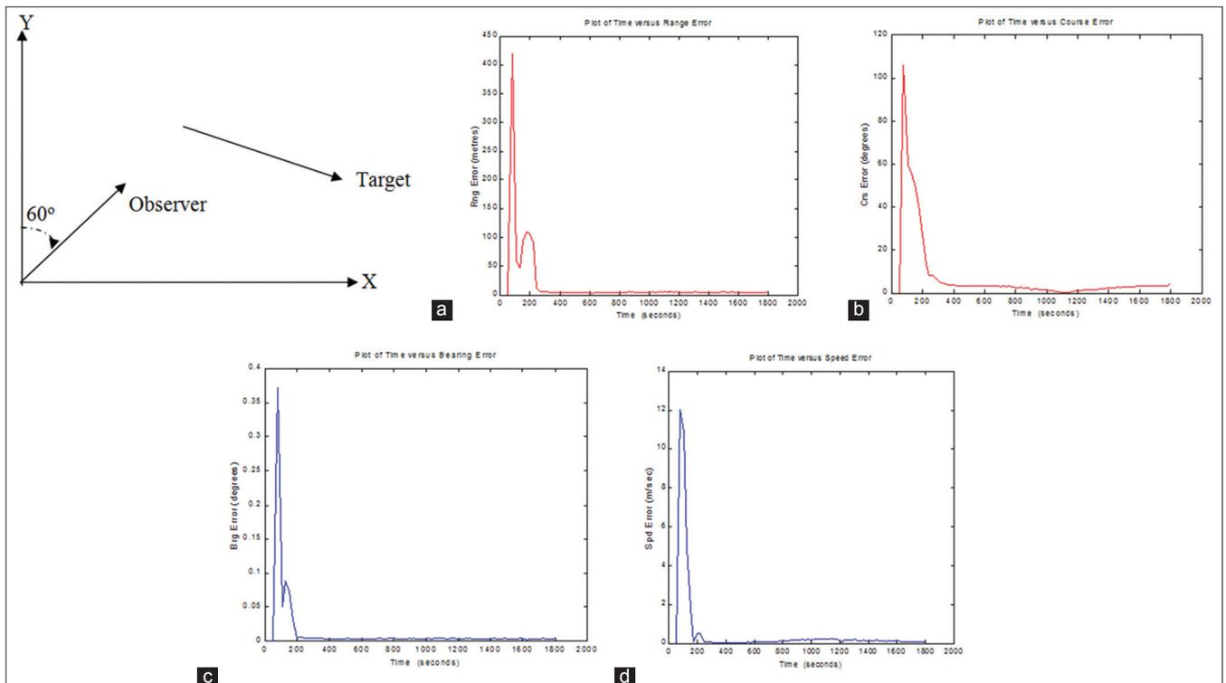
Fig. 2: Target motion analysis with single observation platform with straight run target, (a) Error in range estimates, (b) error in course estimates, (c) error in bearing estimates, (d) error in speed estimates
