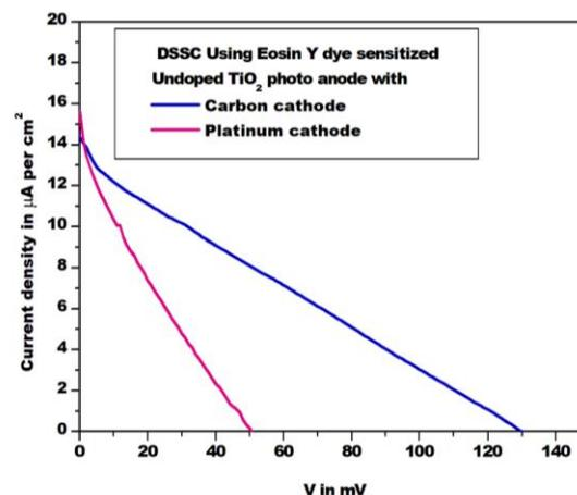
Fig. 2: Photovoltaic characteristics of DSSC- TiO<sub>2</sub> nps photo anode and Platinum and Carbon cathode
