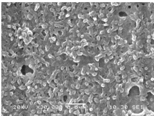
Fig 2: SEM micrograph of PANI-HCl matrix synthesized at 1.0 pH, 0.2 M aniline, 1.0 M HCl T=27 °C.
