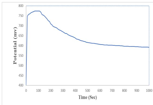
Fig. 1: Potential-time curves obtained synthesis of polyaniline Matrix
