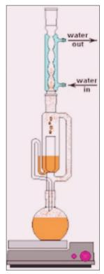
Fig. 1: Soxhlet apparatus to extract beta-carotene [12]
