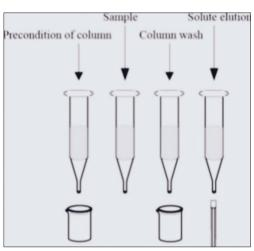
Fig. 2: Solvent extraction to remove impurities [13]
