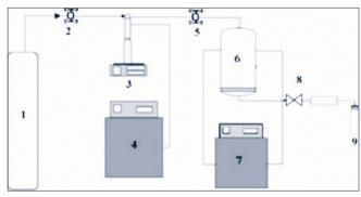
Fig. 3: Propane oil extractor [17]. (1) Propane cylinder, (2, 5) needle valves, (3) high pressure pump, (4, 7) thermostatic bath, (6) extractor, (8) micrometric expansion valve, (9) flaxseed oil collector.
