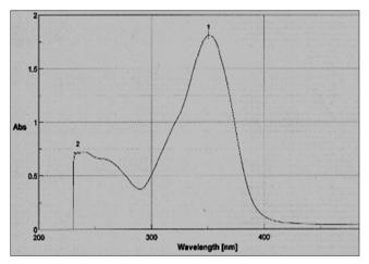
Fig. 2: Ultraviolet-visible spectrum of complex (Zn [L<sub>1</sub>])
