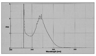
Fig. 3: Ultraviolet-visible spectrum of ligand (L<sub>2</sub>)
