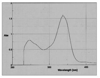
Fig. 4: Ultraviolet-visible spectrum of complex (Zn [L<sub>2</sub>])
